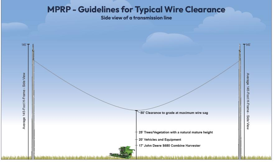
arming and power lines are compatible neighbors. They have co-existed for over a hundred years. The proposed Maryland Piedmont Reliability Project (MPRP) transmission line is designed to provide adequate electrical clearances required by National Electrical Safety Code (NESC) and to be farming compatible in most circumstances.
