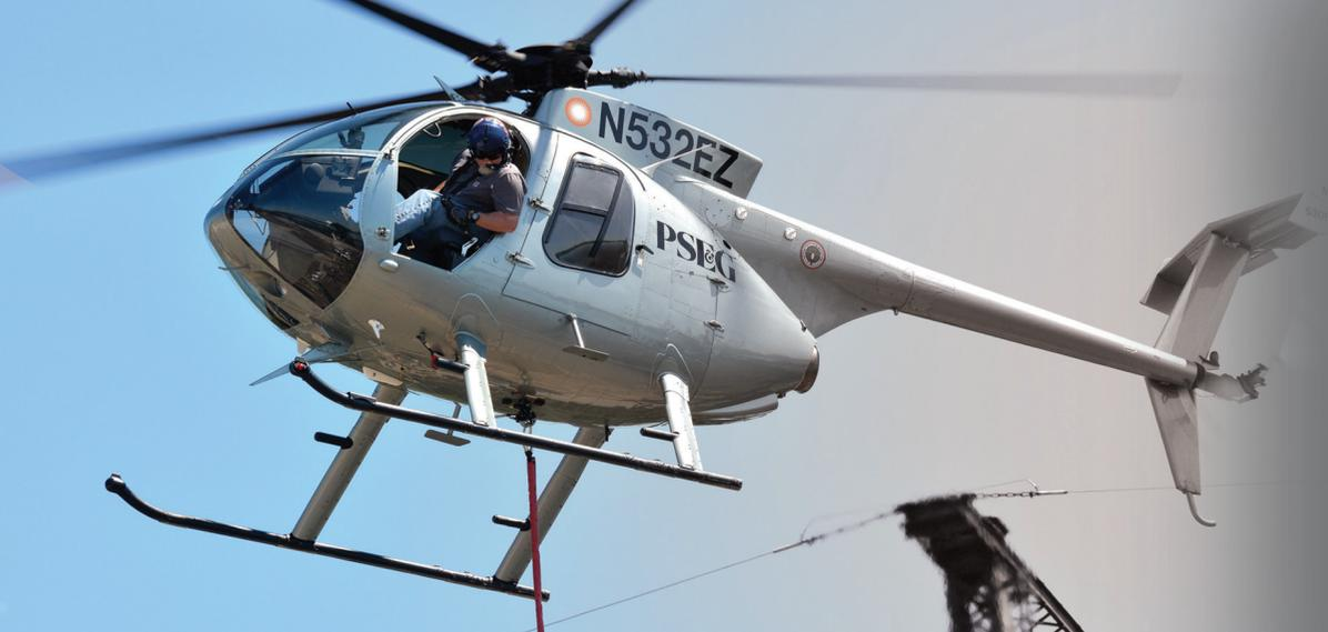
PSE&G uses helicopters in constructing remote portions of transmission lines to minimize environmental impacts. The new transmission lines that PSE&G is building will help maintain and improve electric system reliability for millions of people and thousands of businesses while contributing to New Jersey's economic vibrancy.
